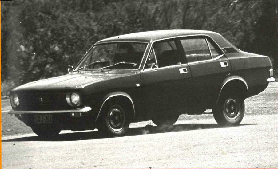
Excessive nose dip accompanies hard braking. Brake fade became pronounced during tests. But despite all, rear wheels never lock.
