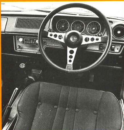
Above: Easily read through the steering wheel, the three-dial instrumentation is fairly basic. Coupe version offers tachometer instead of clock.
